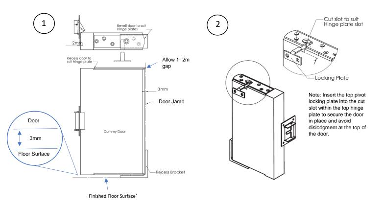
**Safety Warning:** Only install the bottom corner pivot directly onto the finished floor surface. An unsupported bottom pivot is deemed as unsafe for use and may result in flex in the product and dislodgment of the door.
